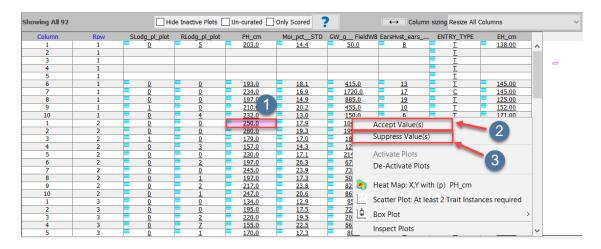
Fig. 2.65: Accepting or Supressing Measurements
